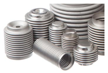
Seamless bellows do have some package size limitations. Their sweet spot for OD lies between 0.25 to 3 inches. Seamless bellows also have a higher initial tooling cost than seam-welded bellows. At production volumes, however, the tooling costs of bellows all but disappear.
