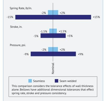
Seam-welding bellows, however, do not lend themselves to applications that require a very precise spring rate. The reason is that their wall thickness tolerances are determined by the sheet metal stock, not the precision deep drawing process. Typical wall thickness variation for seam-welded models is  $\pm$  0.0005 inches, or about five times greater than a seamless bellows.
