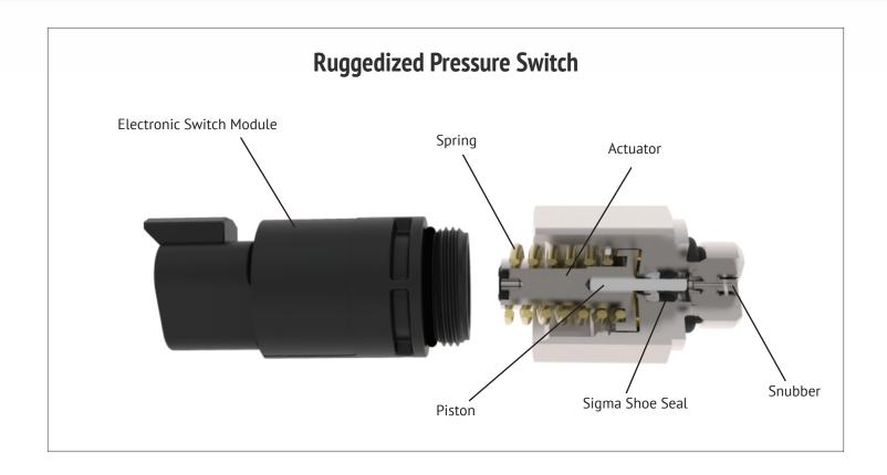
high place enormous stresses on every switch component and represent the most catastrophic failure mode for heavyduty pressure switches.
